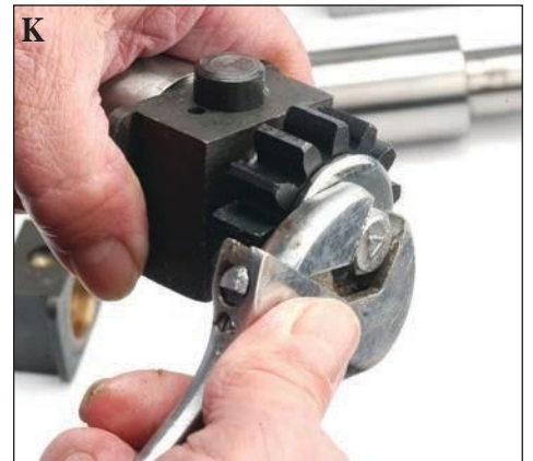
K) Remove the bolt that secures the gear and block to the upper roll.
